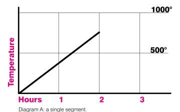
Rate is figured in degrees per hour. In Diagram A above, the temperature takes two hours to reach  $750^{\circ}$ . The rate is  $750 \div 2 = 375$ .
