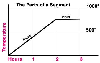
Diagram C: a single segment with hold. The two parts of a segment are the ramp and the hold. Not all segments have a hold, but they all have a ramp.
