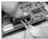
The button-type thermocouple connector: press down, then insert
