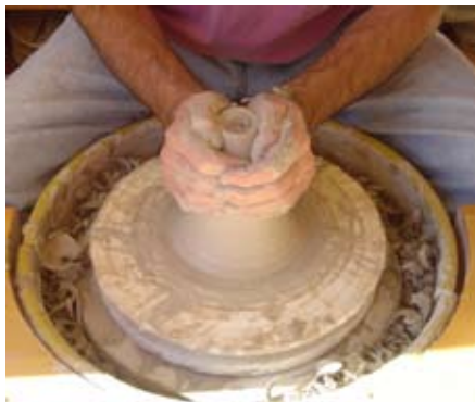
Figure 9. Incorrect concave shape.
