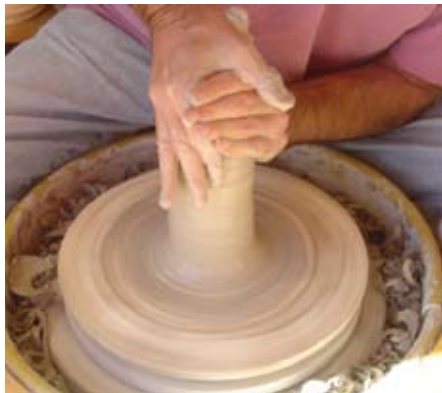
Figure 5. Pushing the cone down.
