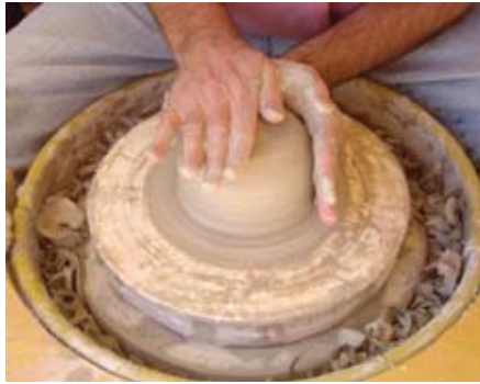
Figure 6. Returning the form to the centered position.
