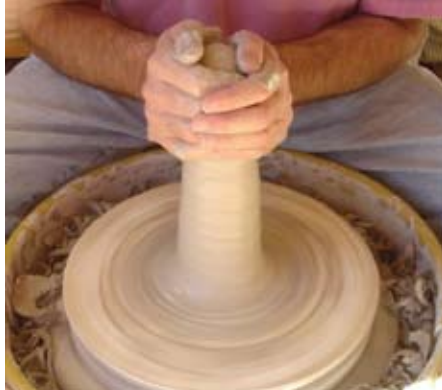
Figure 4. Forming the cone's shape.
