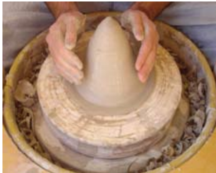
Figure 8. A pyramid indicates incorrect form.
