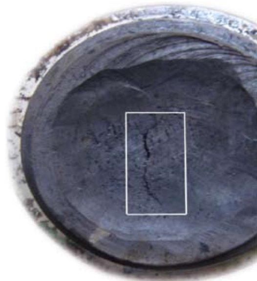
Close-up view of an “S” crack on the inside foot of a thrown pot. Occasionally, the crack can run straight across the bottom of the pot and have a slight curve on either or both ends.
