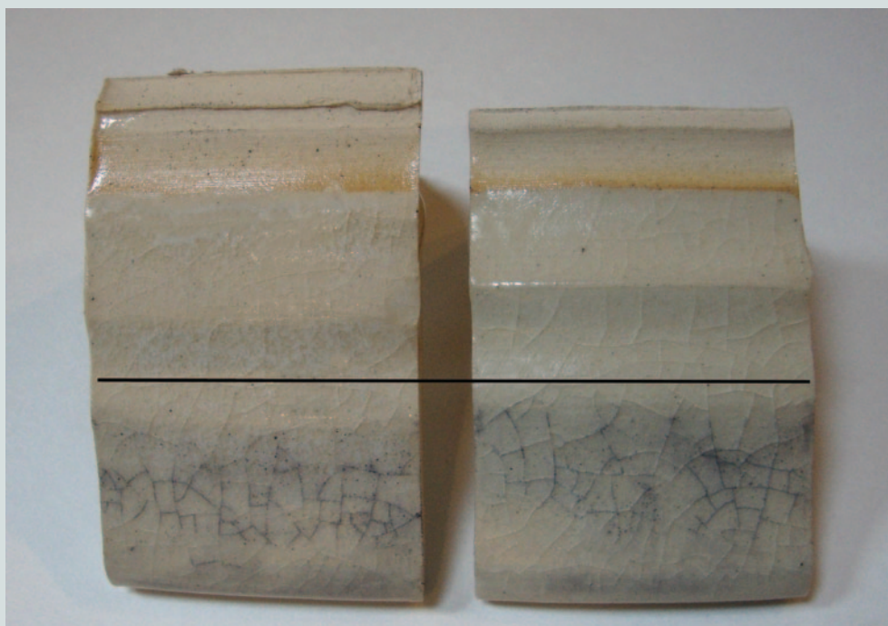
6. Left tile: Transparent gloss glaze using original Cornwall Stone. Right tile: Transparent gloss glaze using new Cornwall Stone.
