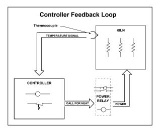
The temperature inside the Kiln is constantly being adjusted by the controller in response to the thermocouple signal.
